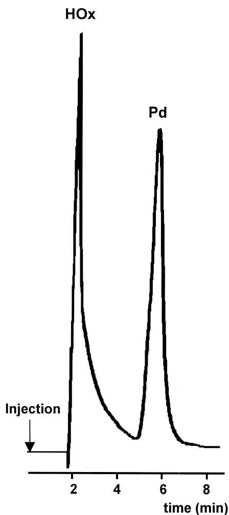
Fig. 2. Chromatogram obtained for a Pd sample (202 ng) with 100% ACN mobile phase in reversed-phase HPLC. Chromatographic conditions: 20 \mu l injection, 1.0 ml min -1 .
